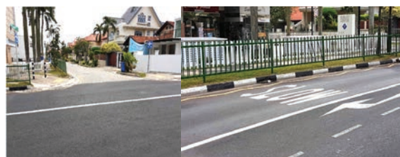
13 Widened Footpath at junction of Burnfoot Terrace and Siglap Road with additional measures of "SLOW" Road Markings along Siglap Road and Painted Chevrons on both sides of Burnfoot Terrace
